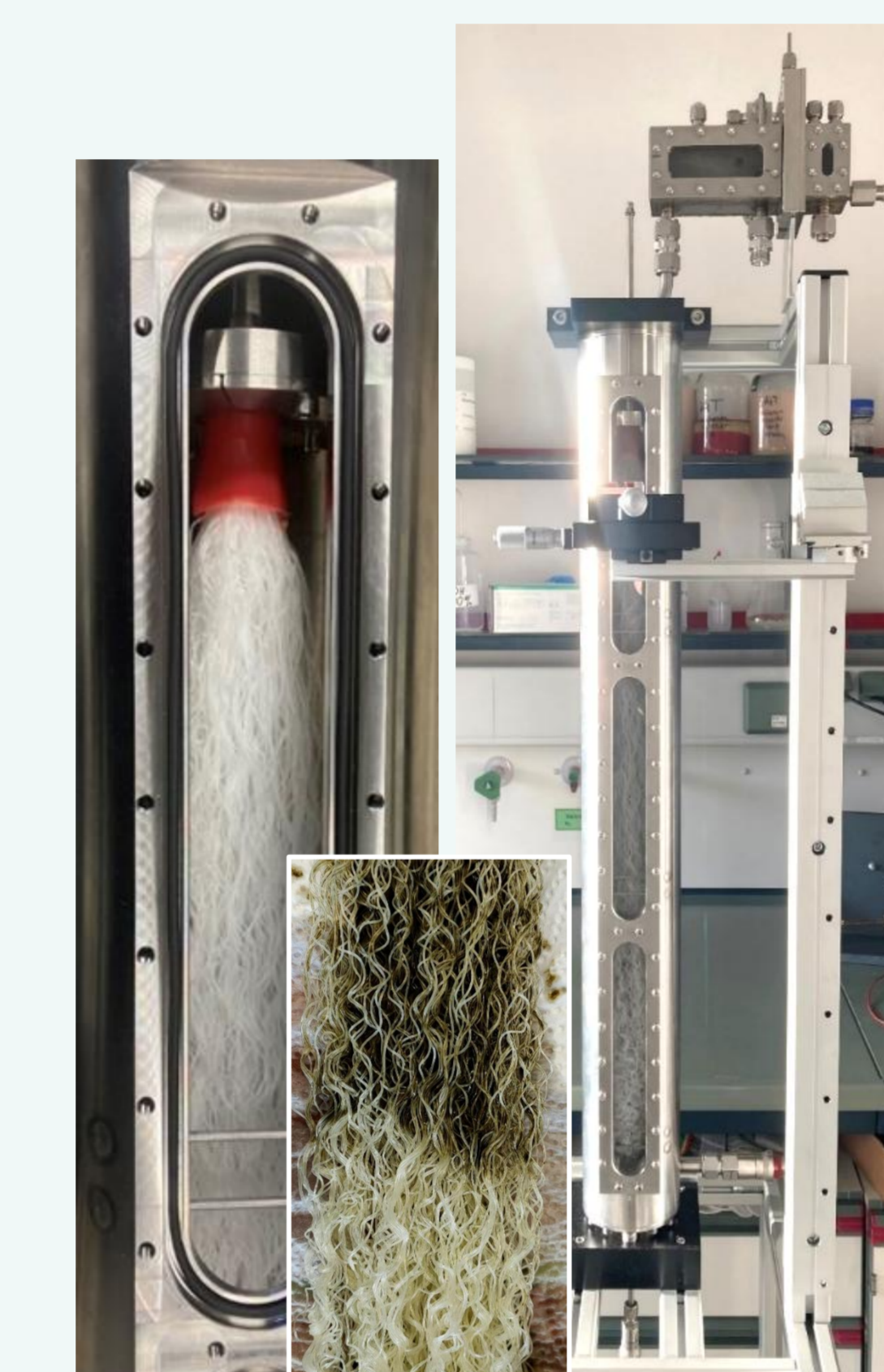
MBfR with dense silicone hollow-fibre membranes (left: bare, middle after months of cultivation)
